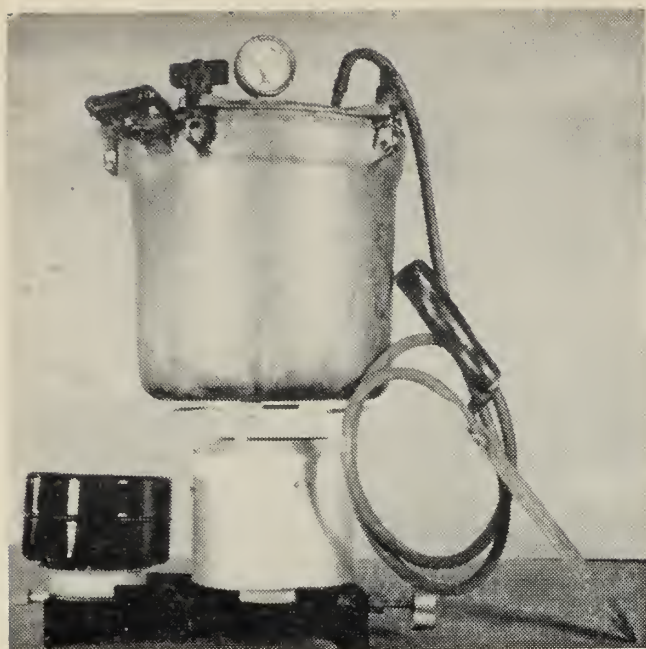
A handy source of steam for a single uncapping knife.
