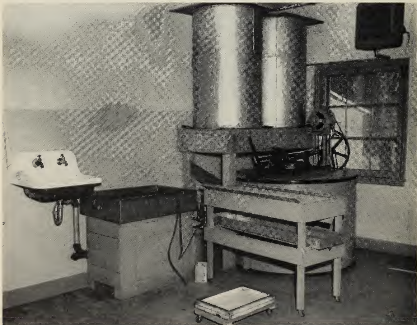
A compact arrangement of honey extracting equipment. The cappings are melted in the steam-jacketed cappings melter and the honey and wax separated as they run out. The uncapped frames are stacked in the comb table while the honey extractor is operating. The honey is pumped from a sump to the tanks. Steam comes from a boiler in the small building seen through the window.
