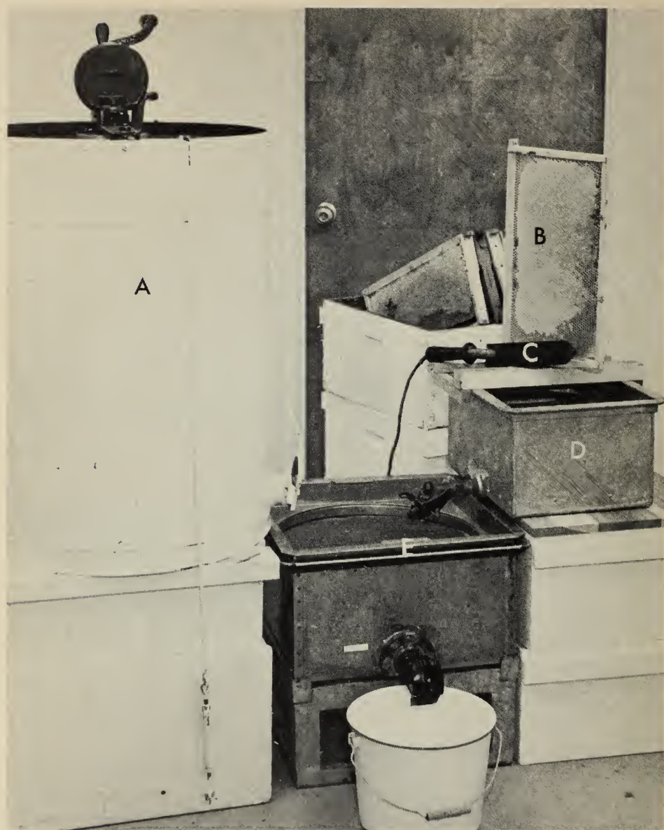
Working set-up for extracting small quantities of honey. A: 4-frame extractor; B: frame of honey ready for uncapping cells; C: electric uncapping knife; D: box with strainer to collect cappings and honey; E: sandwich-type filter for final straining. Four frames yield about 20 pounds.
